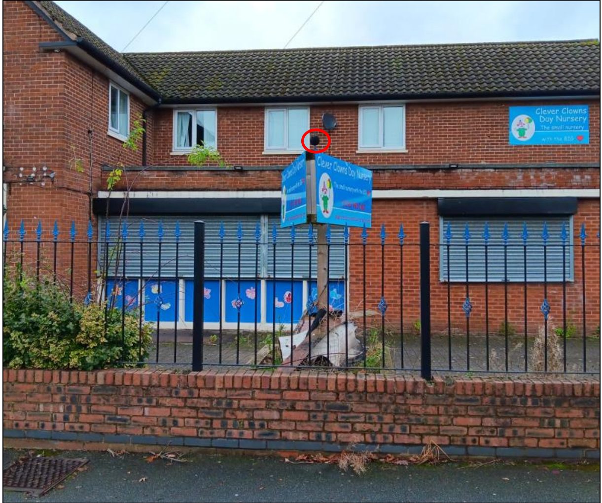
Figure 5: Photograph of meter in position (microphone circled)
