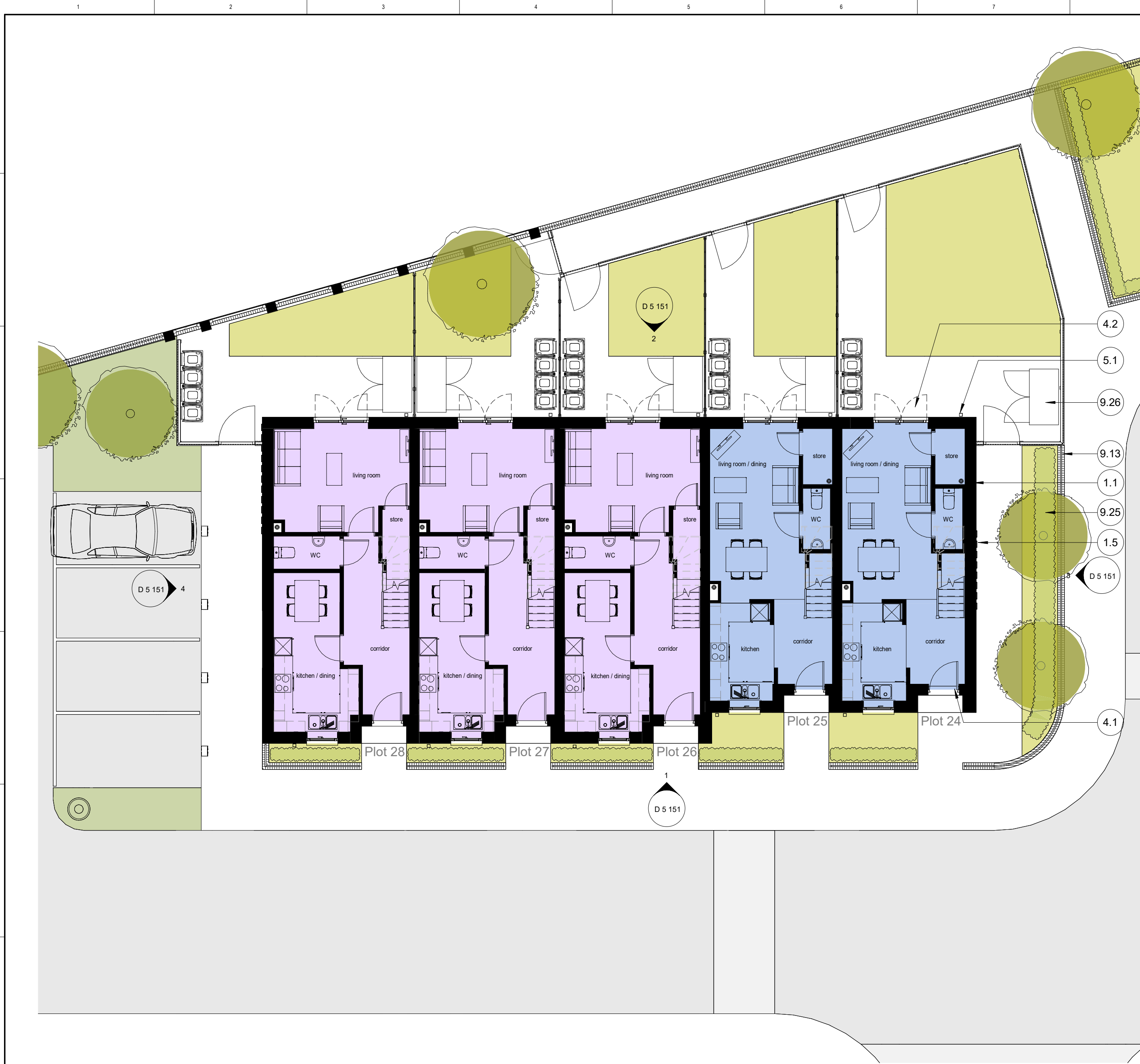
1 Building 5 Ground Floor Plan 1:100
