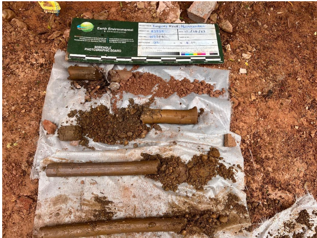
View showing the two monitoring installs, one for shallow 1m vapour installation and a deeper groundwater installation
