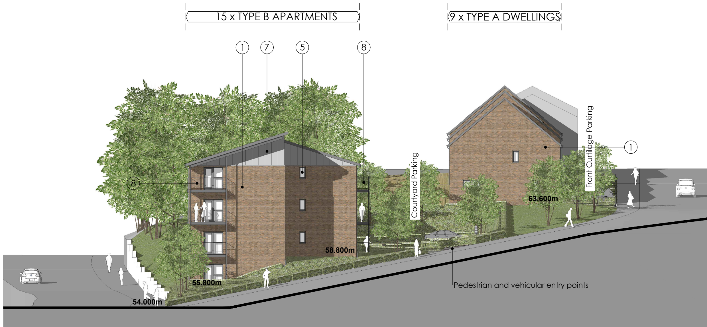
Street Elevation 3: North-East Facing Cleveland Road Elevation:1:200
