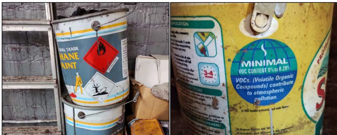
Figure 8: Photographs showing the 'flammable' and 'harmful to the environment' hazard labels (left) and VOC content label (right) on eroded paint tins located in the basement.
