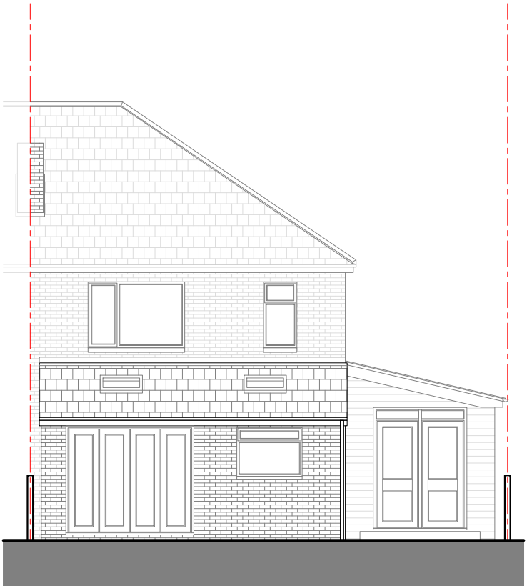
EXISTING REAR ELEVATION 1:100 @ A3
