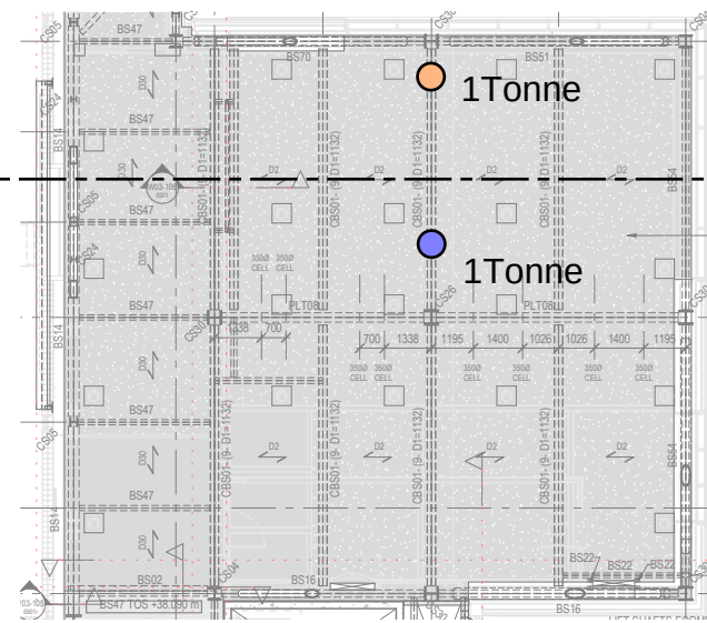
Scenario 1 - 2 x 1 Tonne applied to the same beam
