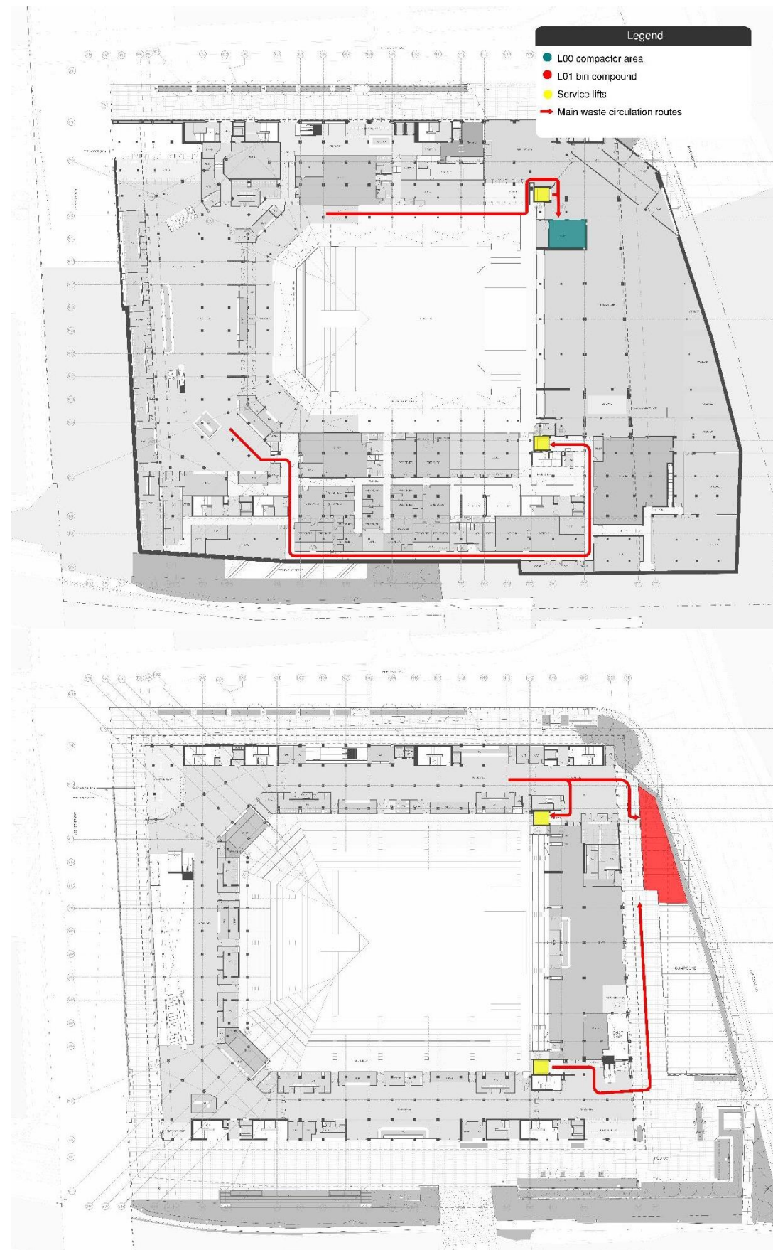
Figure 3.4 Illustration of main waste movement routes (ground floor and L01)
