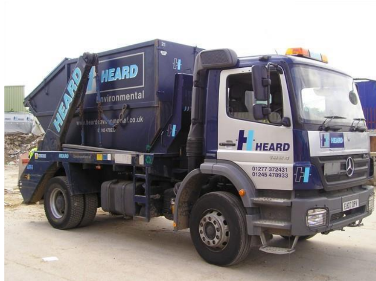
Figure 3.8 Example of skip-lift swing-arm truck
