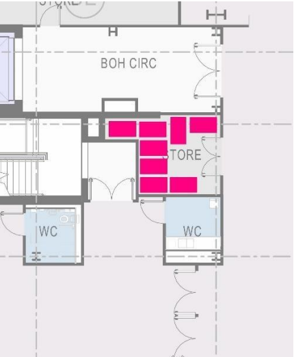
Figure 4.1 Indicative layout of potential L03 intermediate waste store
