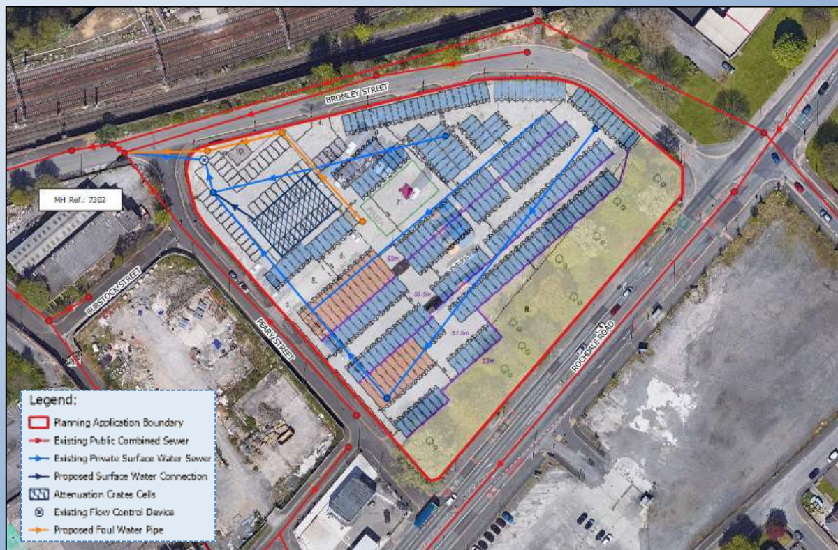
Figure 6: Preliminary Drainage Strategy (Betts Hydro, 2023)
