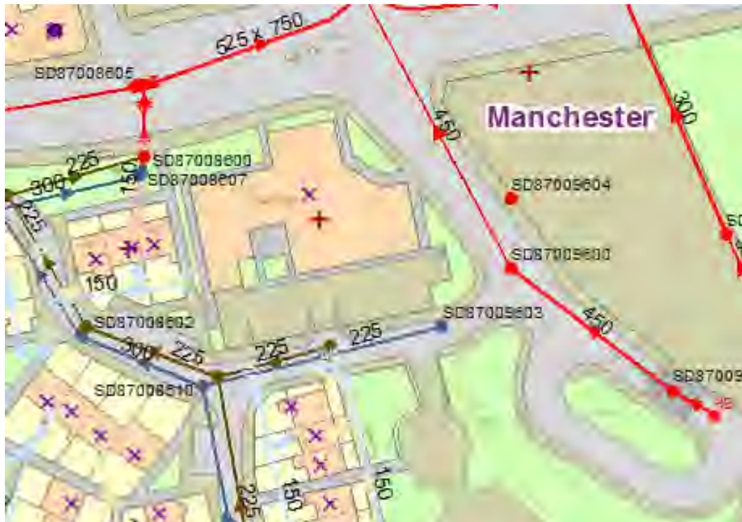
Figure 3: United Utilities Public Sewer Extract 2023
