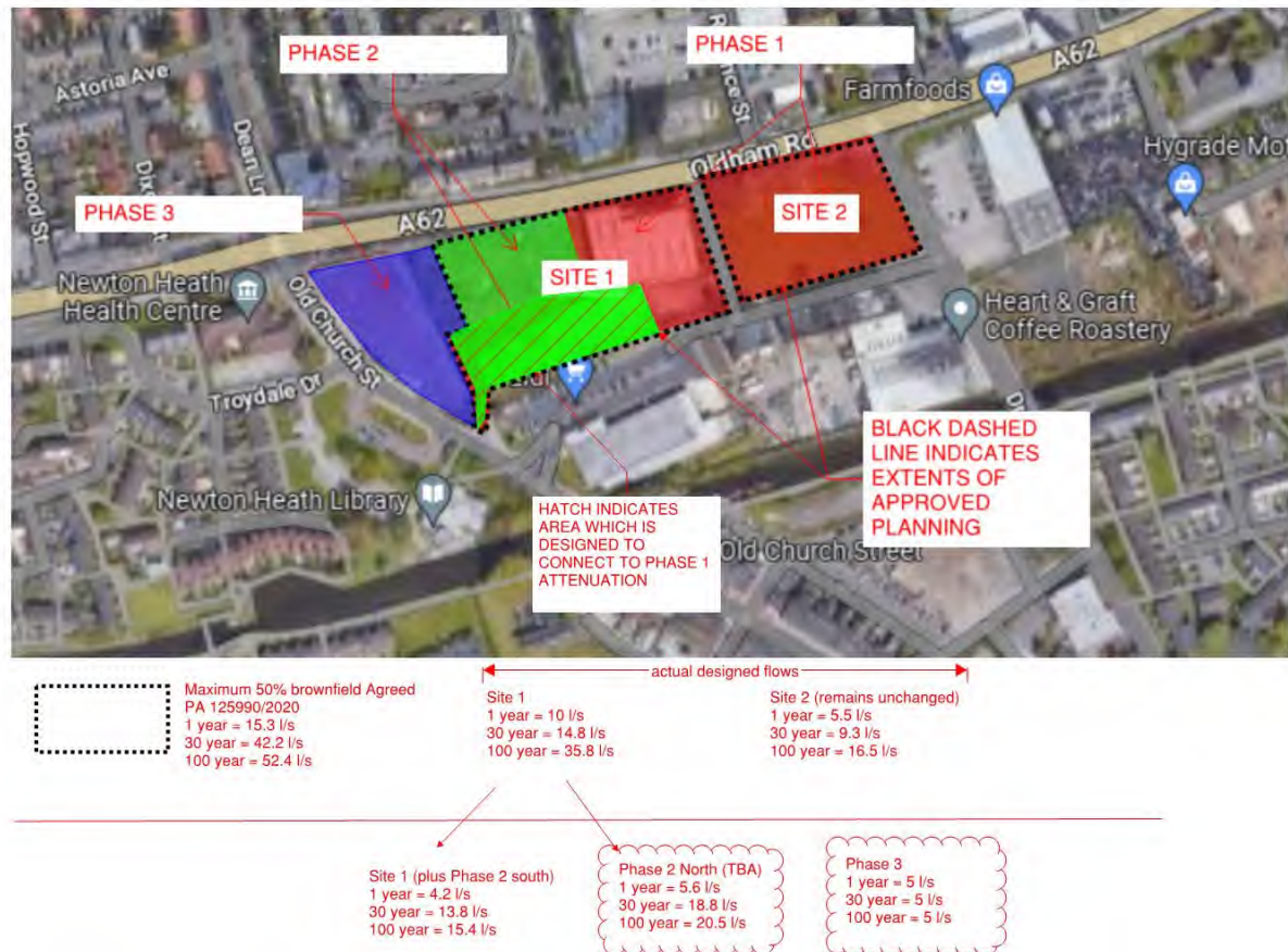
Figure 10: Phased Development Surface Water Flows
