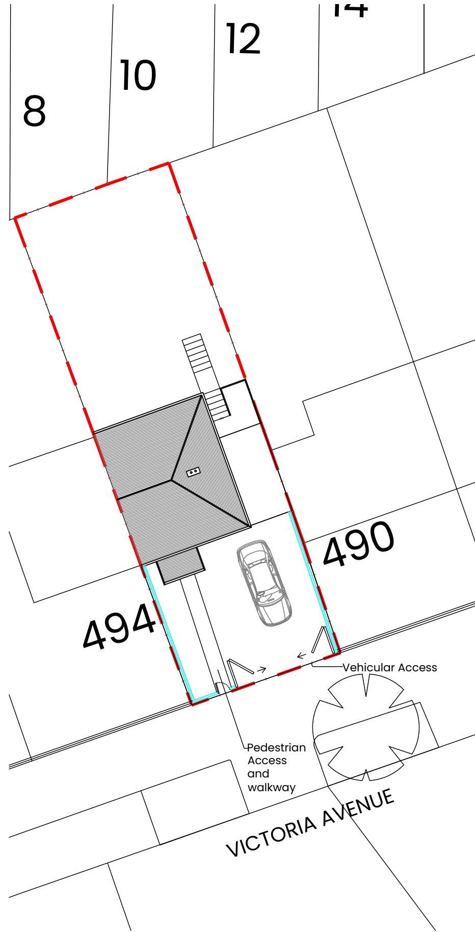
03 As-Built Boundary Treatment Site Plan Scale 1:200 @ A3
