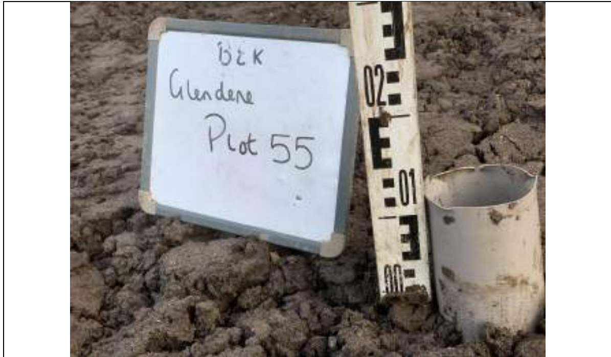
Photograph 3: Validation of Garden Capping
