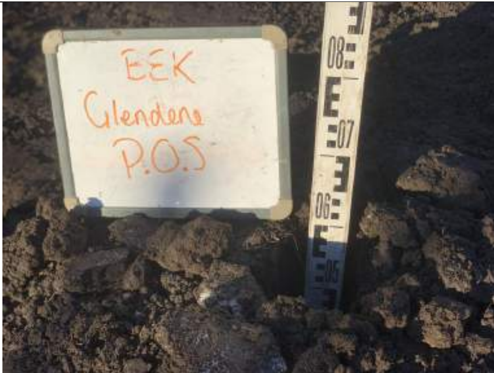
Photograph 3: Validation of Public Open Space Capping
