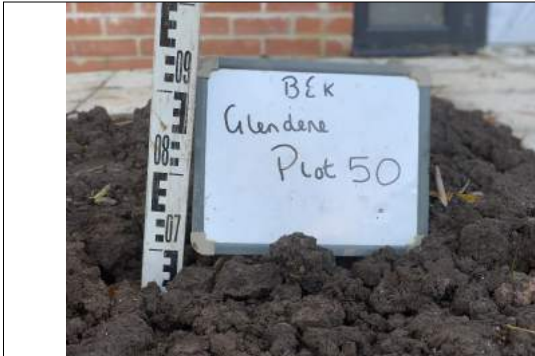
Photograph 1: Validation of Garden Capping
