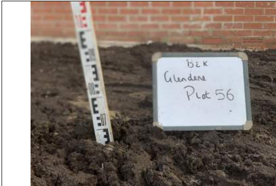
Photograph 1: Validation of Garden Capping
