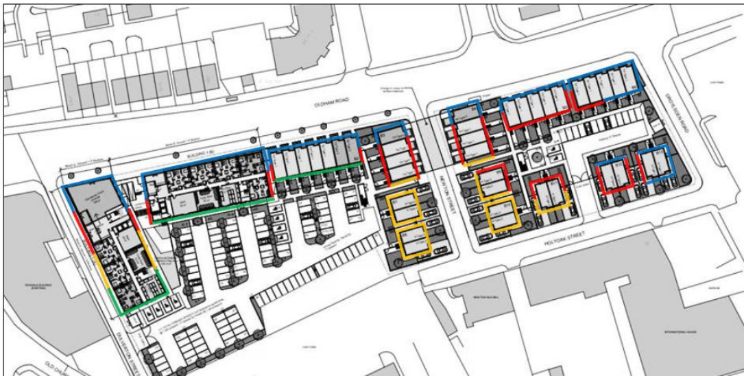
Façade sound insulation performance zones
