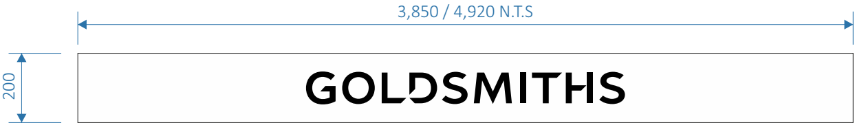
Item B: Fascia Letters- Scale 1:15 2-off Digitally Printed Opaque Vinyl Patches. Note:- Applied to Awning Valance.
