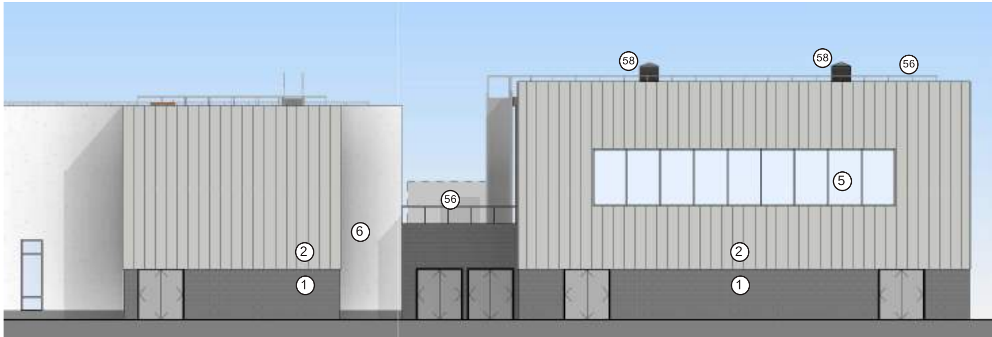
Sports Hall North East Elevation - Standing Seam Cladding
