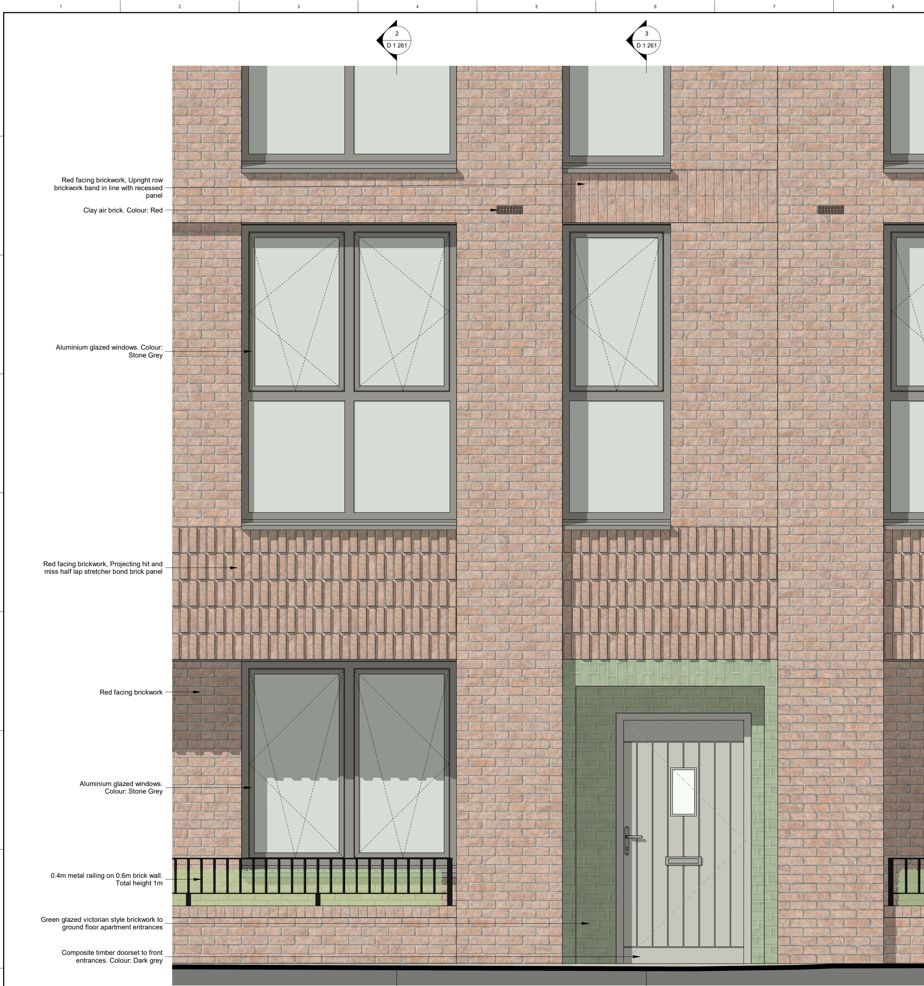
1 Typical Block A Facade: Elevation 1:20
