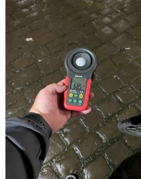
Lux level 68.5 at reference point B (Interference from neighboring light)
