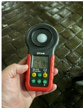
Lux level 5.18 at reference point C
