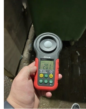
Lux level 20.1 at reference point H (Partial cast off neighbouring light)
