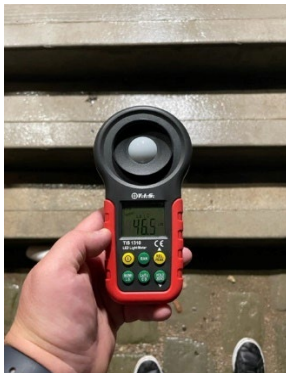
Lux level 46.5 at reference point I (Partial cast off neighbouring light)
