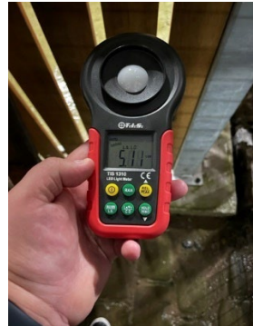
Lux level 5.11 at reference point D
