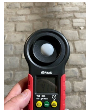
Lux level 42.7 at reference point L (Neighbouring light over powering ours)
