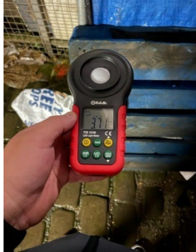
Lux Level 3.71 at reference point A
