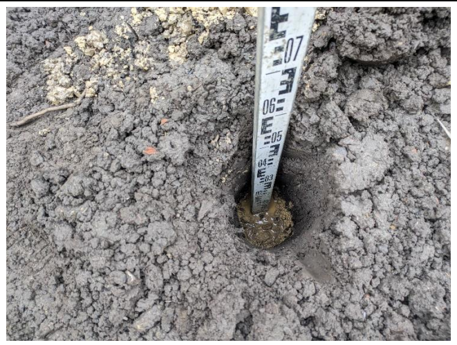
Hand dug pit HP1: Internal view of excavation
