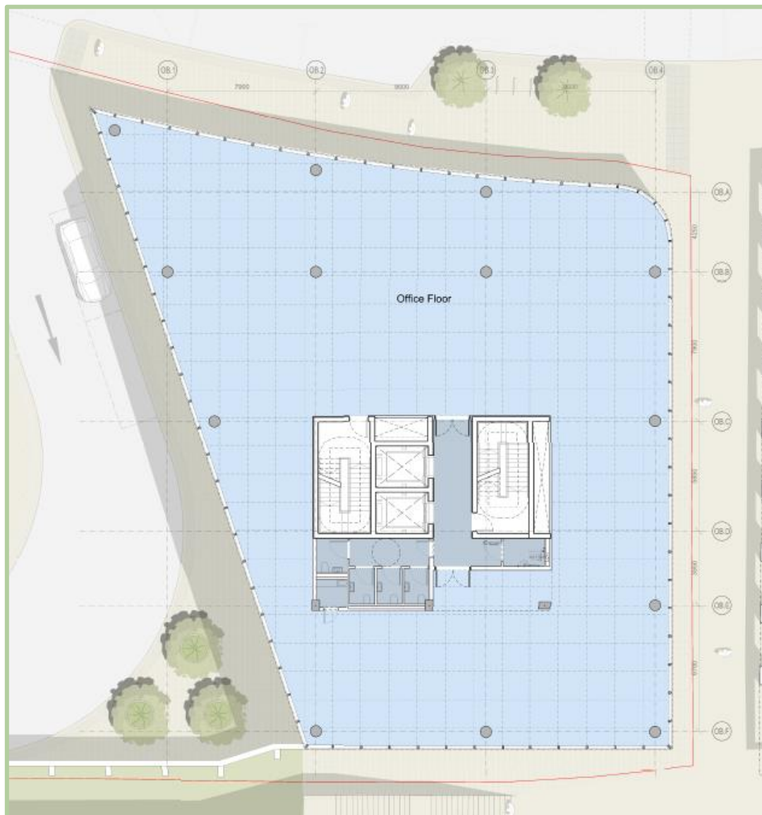
Figure 2.16 – General Arrangement Plan Level 01– Office Block
