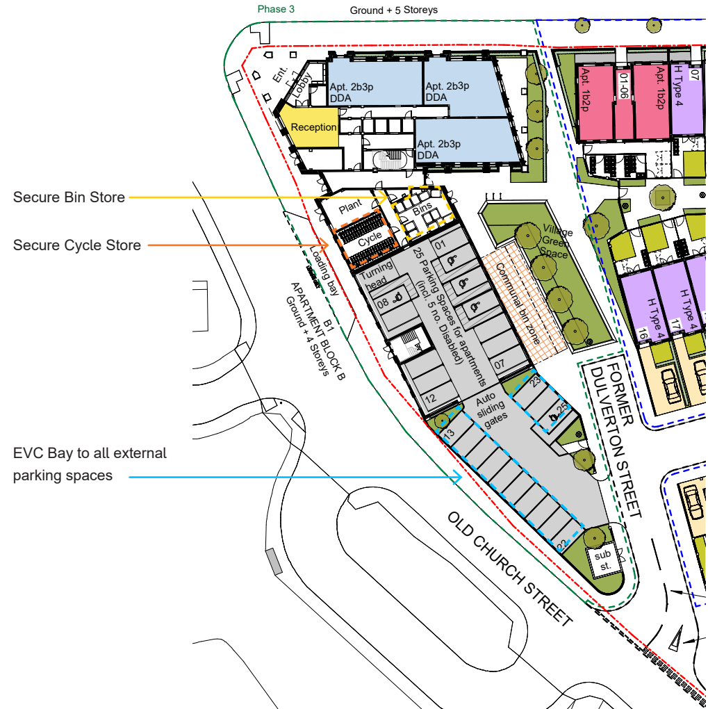
Apartment Building Cycle Store & EVC Parking Bay
