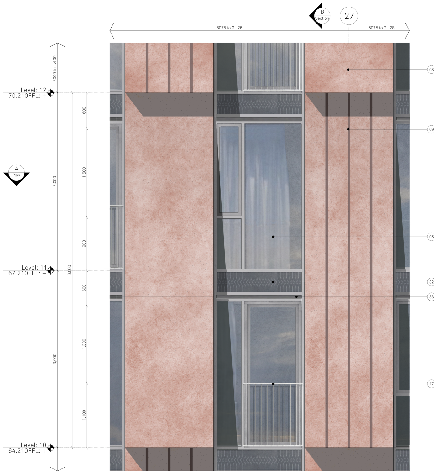
ELEVATION A Typical Bay
