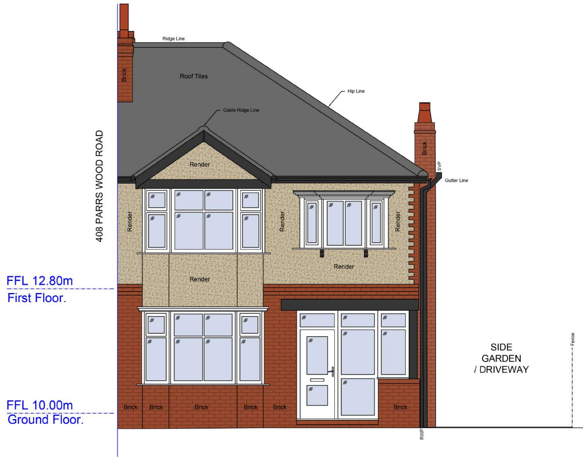
Existing East Elevation - to Parrs Wood Road
