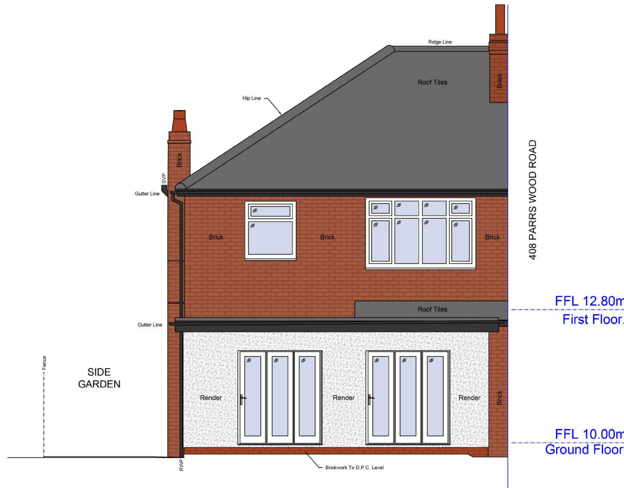
Existing West Elevation - to garden
