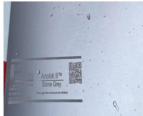
Light Grey anodised cladding - Anolok II - Stone Grey (as agreed on site 19/07/2023)
