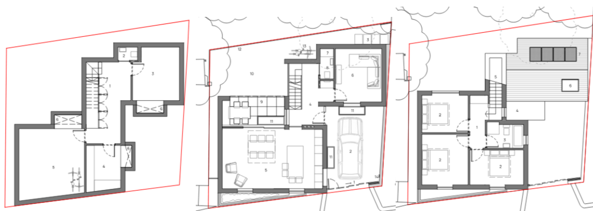
Fig.3 – Internal layout – Basement, ground and first floors.
