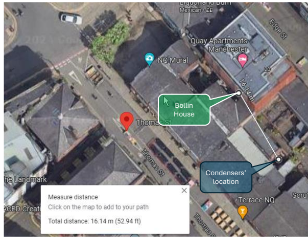
Figure 13 Condenser location in relation to nearest sensitive receptor
