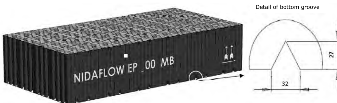
Figure 1d – basic block NIDAFLOW EP grooved on 2 sides
