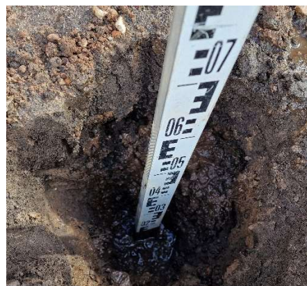
Depth of pit demonstrated at 600mm
