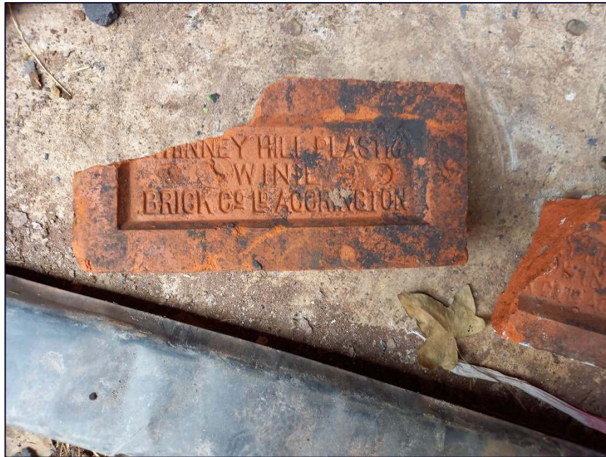
Plate 13: Frogged brick removed as part of current work. Stamped “Whinnney Hill Plastic Winil Brick Co. Ltd Accrington”
