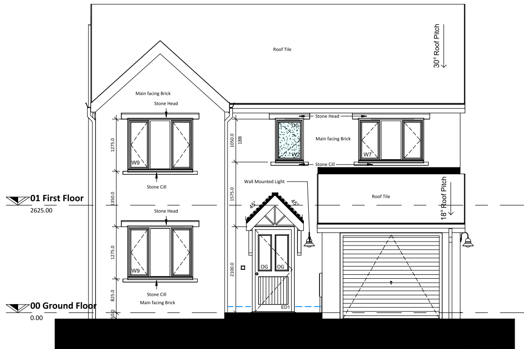
Existing Front Elevation S/O 1 : 50
