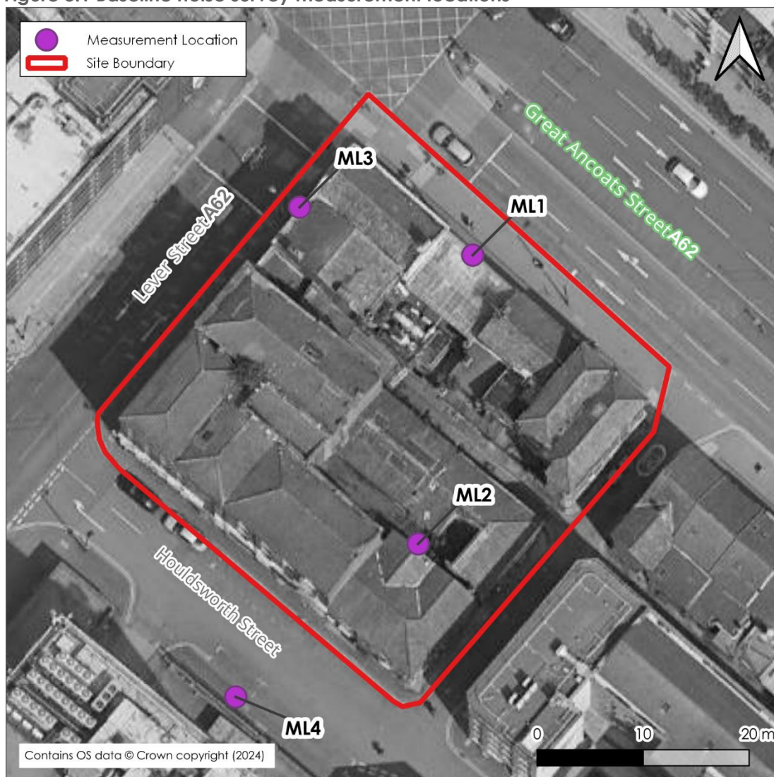
Figure 3.1 Baseline noise survey measurement locations
