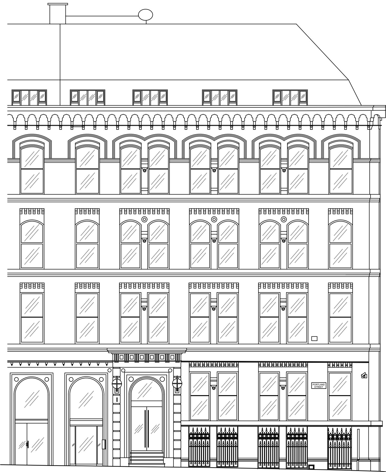
01 ELEVATION A-A PROPOSED REPAIRS 130 SCALE - 1:100 @ A1
