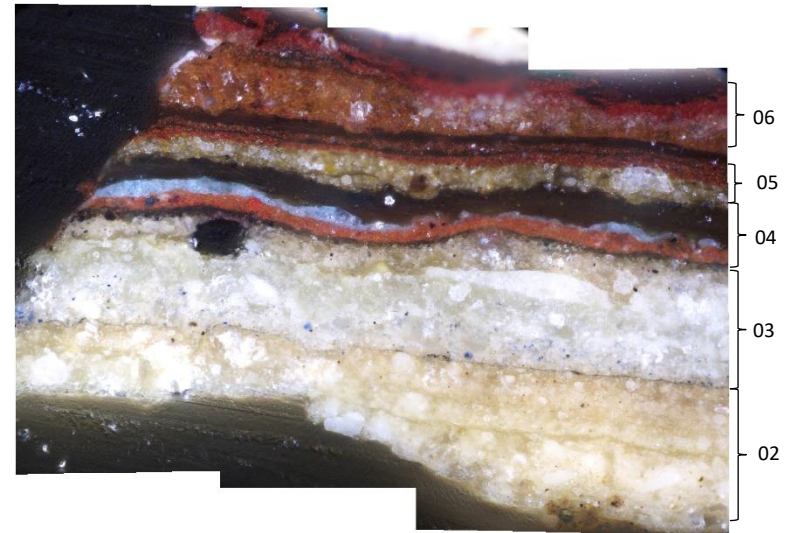
Figure 19: sample 03 (taken at 500x magnification, brightfield mode) showing the composition of layers in the earliest schemes of decoration.
