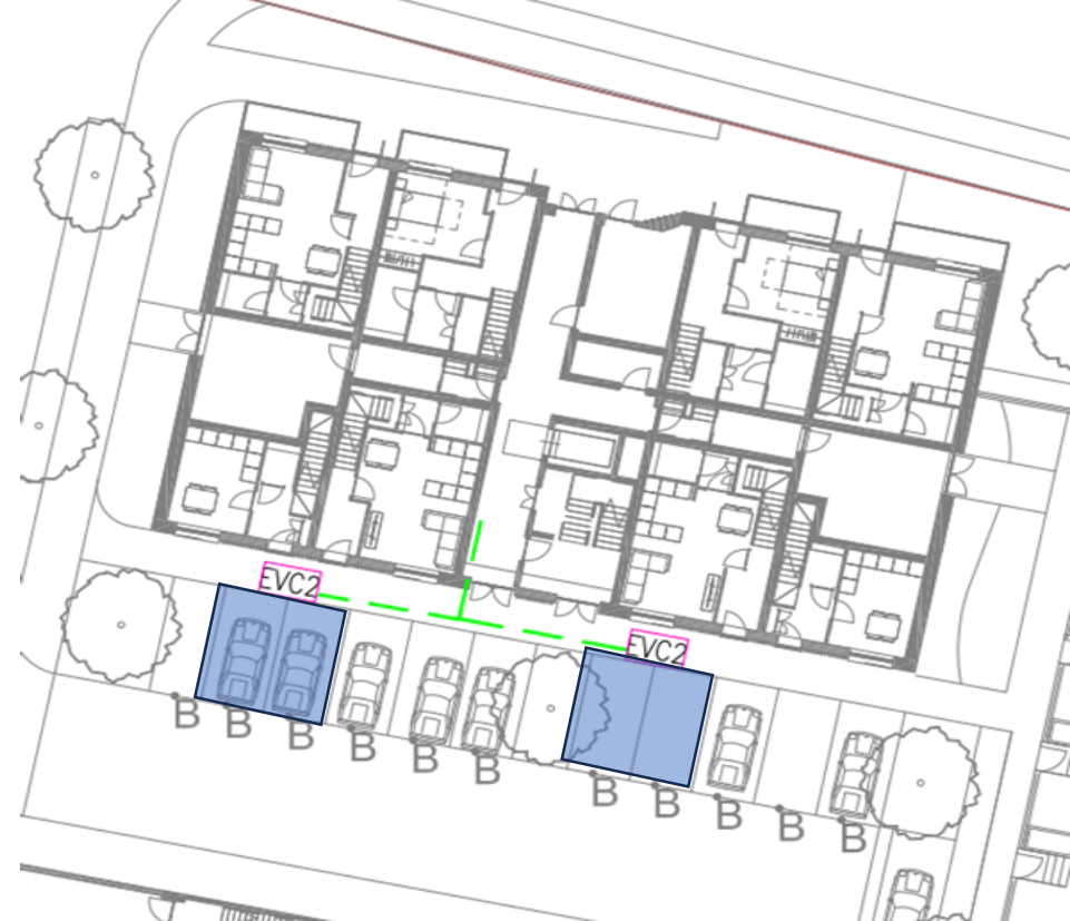
Apartment Block 2 (C1) – Charging Points – 4 x Car Parking Spaces
