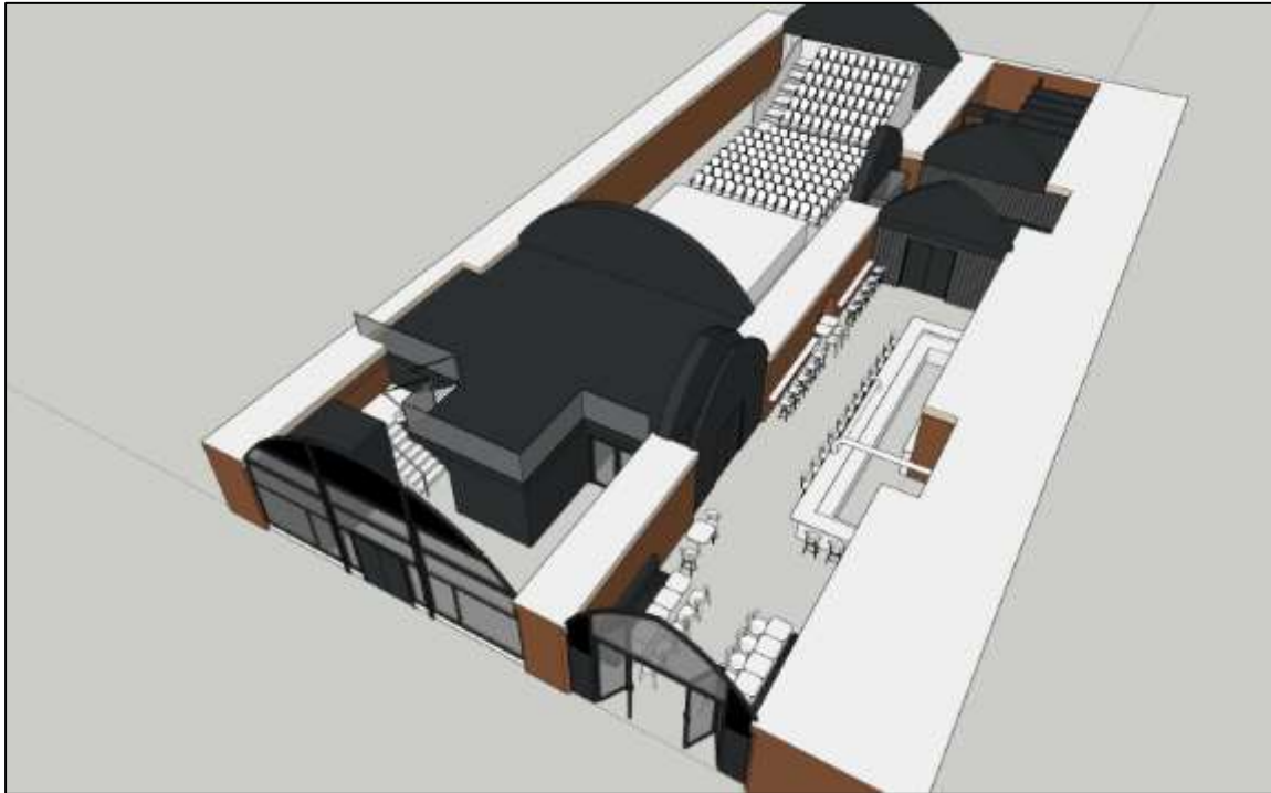
Figure A: 3d Image of the proposed development. Illustrating the plan form of both Arch 18 (Theatre, left), and Arch 19 (Bar, right). The glazed doors which will replace the 1980s brick infill are depicted on the plans. The doors which will reinstate access between the two arches are also shown.
