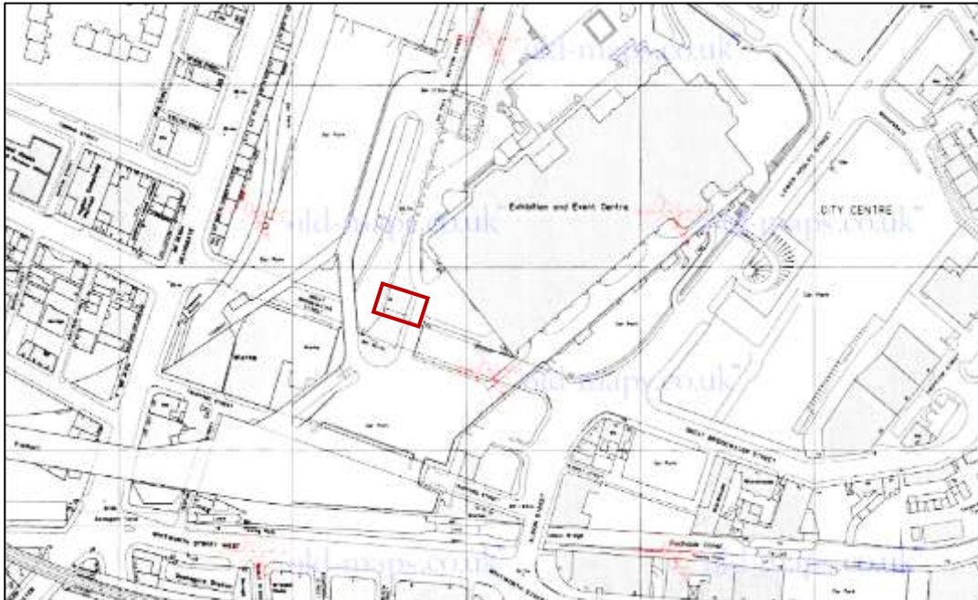
Figure 14: By the late 1980s the area had been substantially altered, following the conversion of Central Station into the new GMEX Convention Centre. This saw the demolition of original entrance buildings and the removal of original track beds to allow for access to the rear of the train shed. The undercroft Site remained unaffected by the new development. Source: Oldmaps.co.uk.
