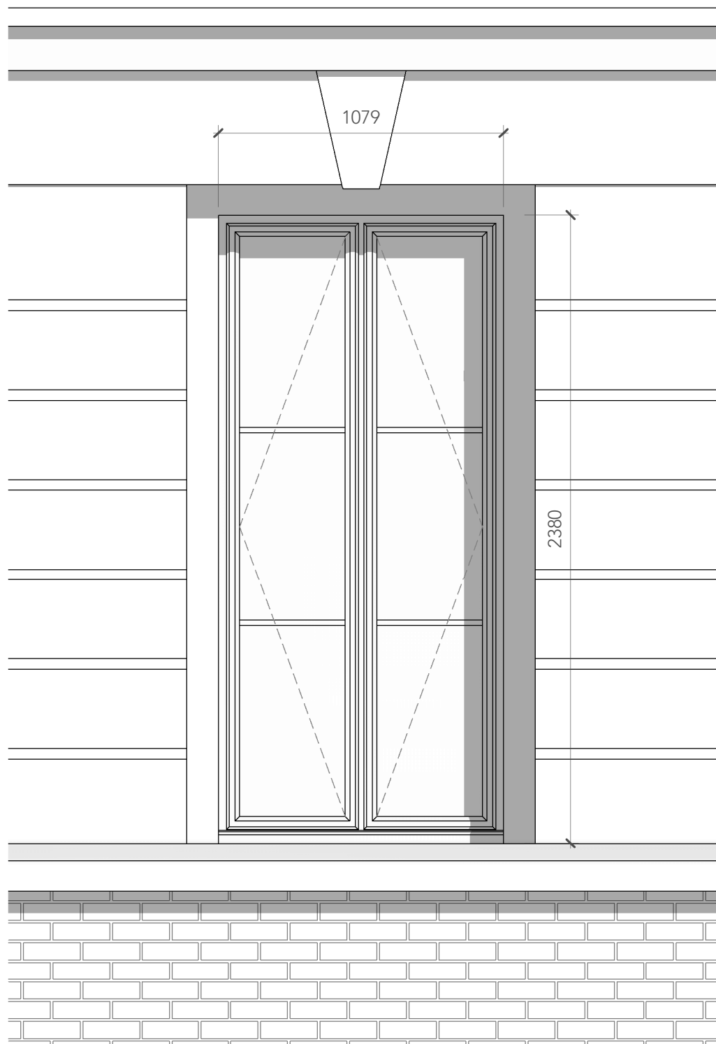
3 Windows_External Elevation WIN-010 and 022 as Existing
