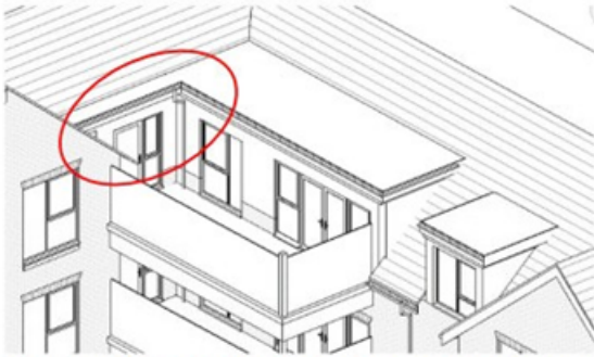
Figure Ten: Previous roof layout showing eaves protruding over balcony.
