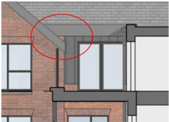
Figure Twelve: Previous Eaves design shown protruding over balcony.
