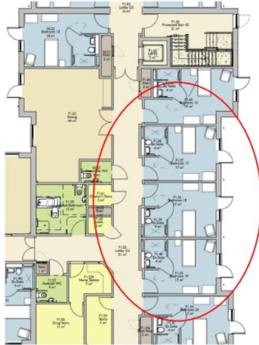
Figure Four: Revised Floor plan with slightly wider bedrooms and stair core relocated.
