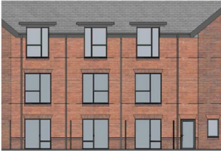
Figure Five: Previous East elevation showing access door leading from stair core and bedroom windows positioned unequally.
