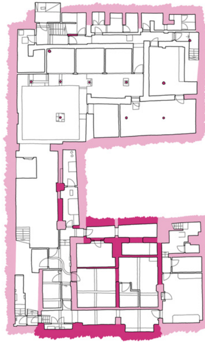
3.112 Basement, suggested survival of fabric existing by 1913
