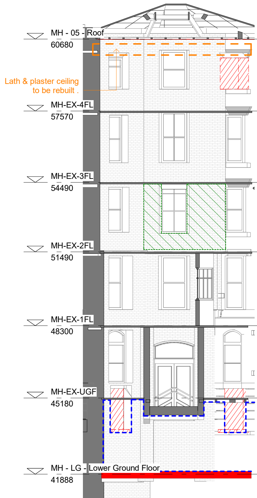
N REMEDIAL INTERNAL ELEVATION. 1 : 100
