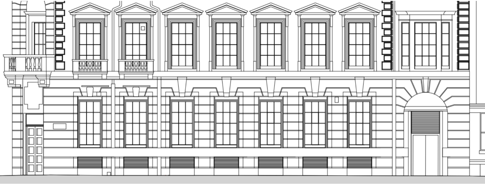
Revised Proposal showing full Chatham Street elevation (ground and first floors) with changes to window openings and retention of stone piers to form the secondary entrance in the arched opening.
