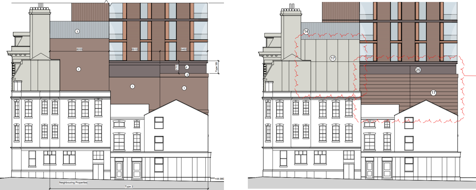
West elevation, submitted drawing (left) and revised proposal (right).
