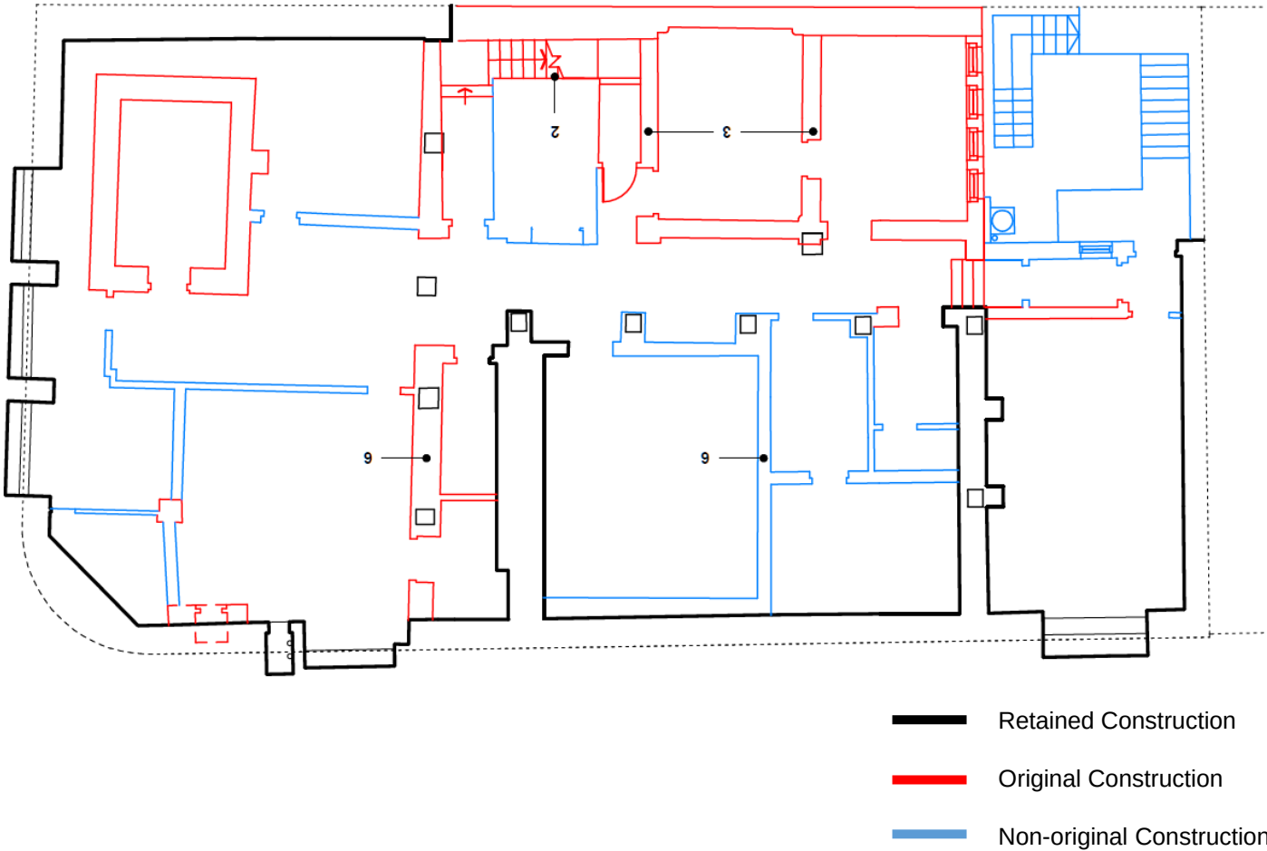
Proposed basement existing / demolition drawing
