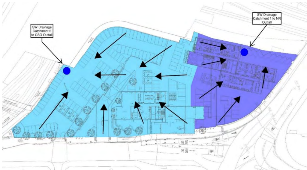
Figure 1 - Surface Water Drainage Catchments
