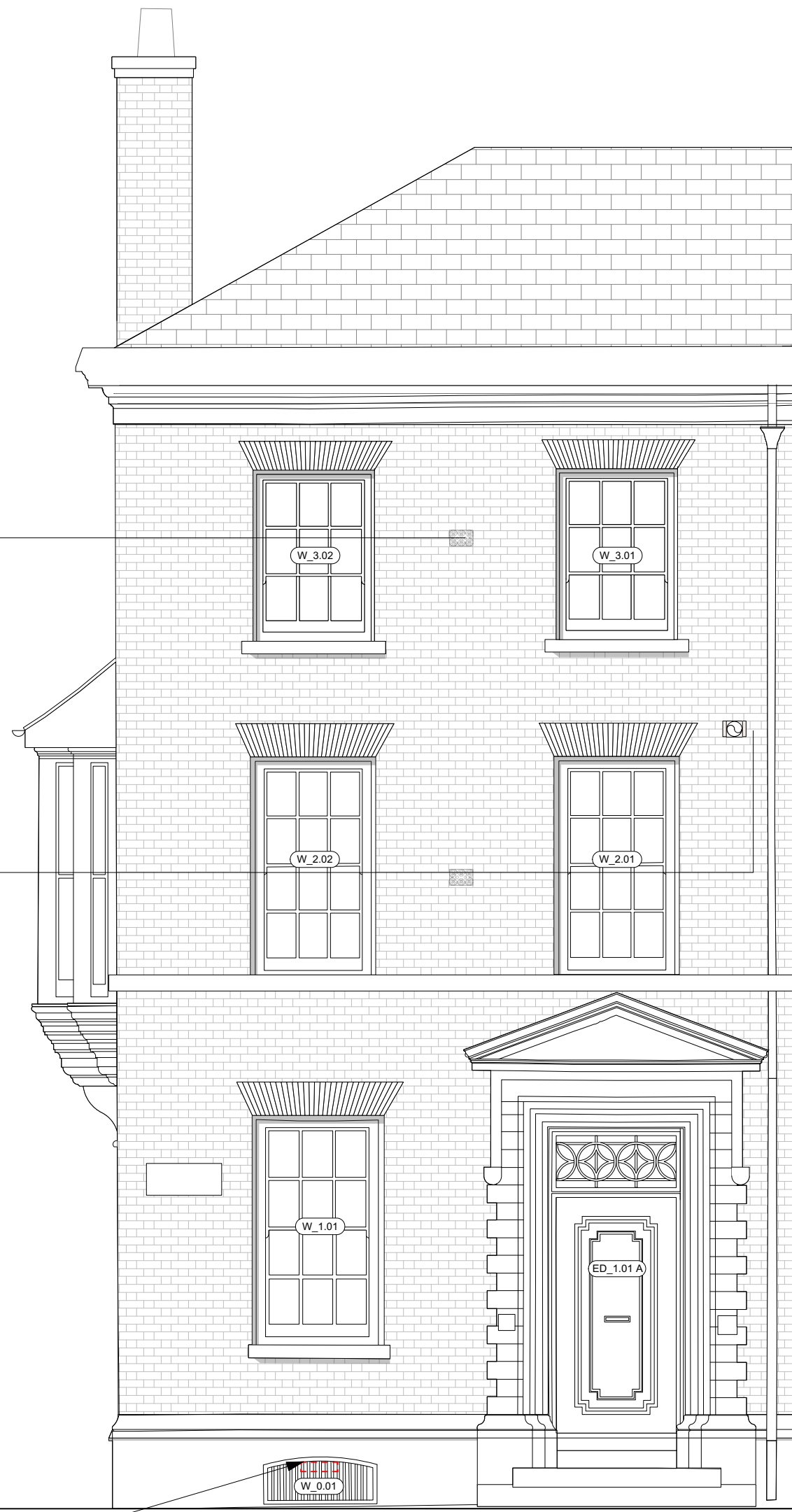
PROPOSED NEW VENT POSITIONS AT GROUND FLOOR AND ABOVE TO EXTERNAL WALL TO MAKE USE OF RECLAIMED CLAY VENTS TO EXACTLY MATCH EXISTING, AVAILABLE FROM: www.authentic-reclamation.co.uk/stock-item/reclaimed-decorative-air-bricks
