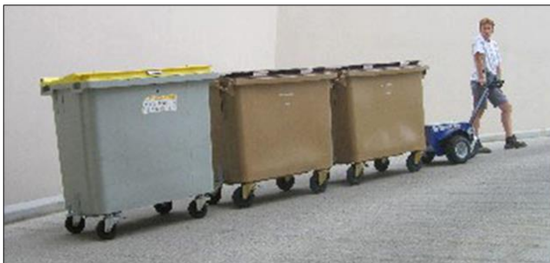
Figure 6.4: Eurobin Powered Pulley System
