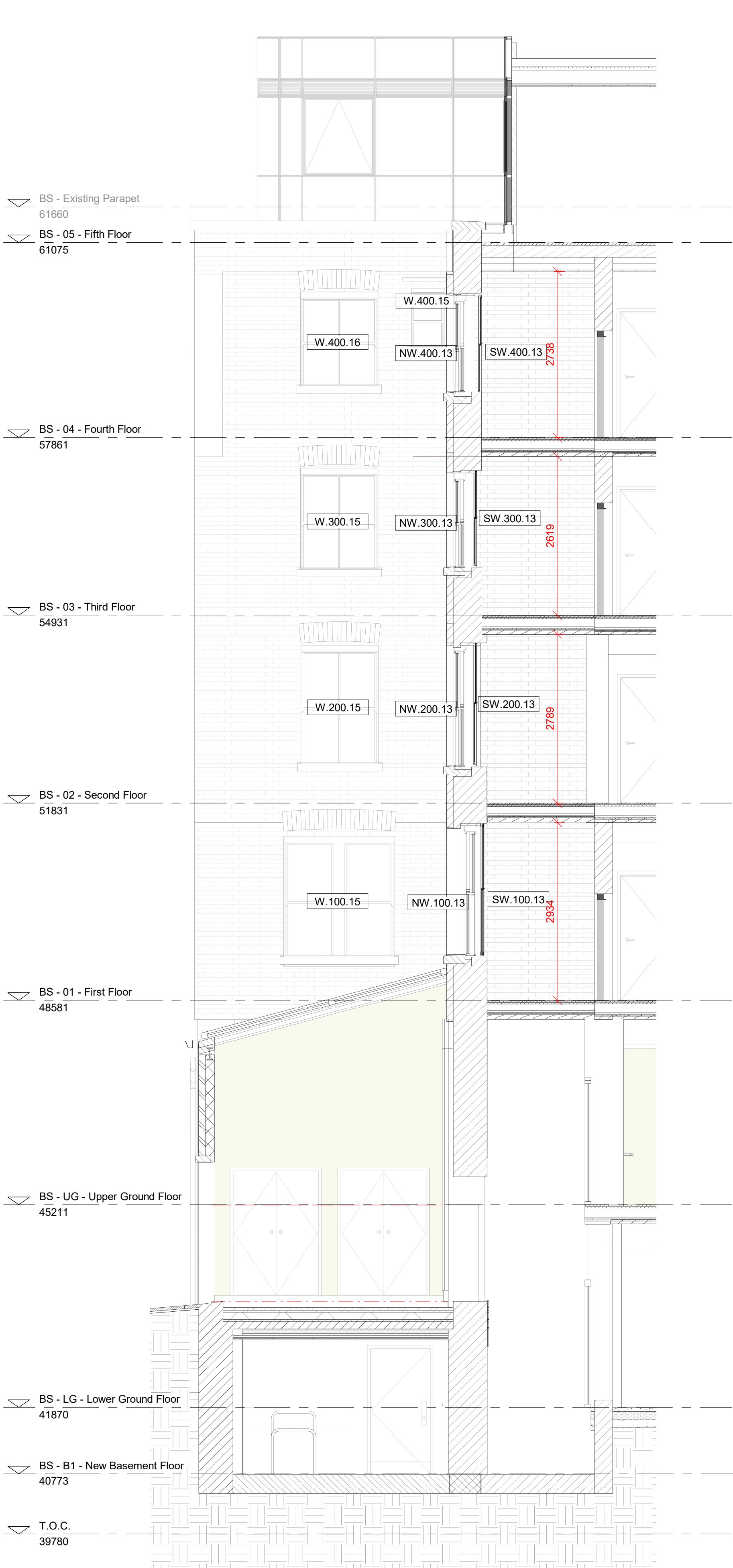
1 EXTERNAL WALL SECTION - ALLEYWAY. 1 : 50
