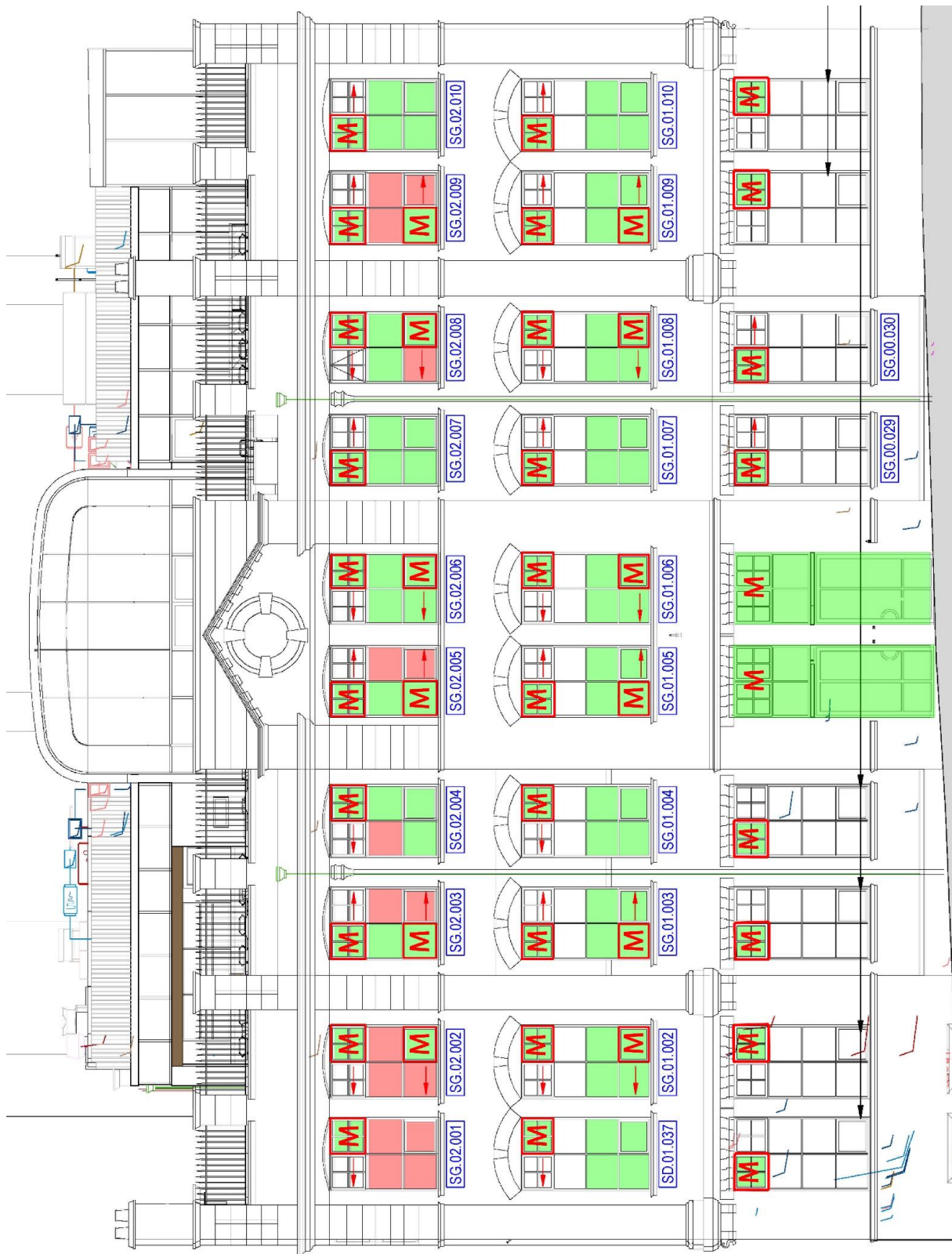
Figure 7: South elevation. Key - Pink (presumed original) Green (presumed replacement) no colour (inaccessible) red outlines and letter “M” (modern timber window unit).
