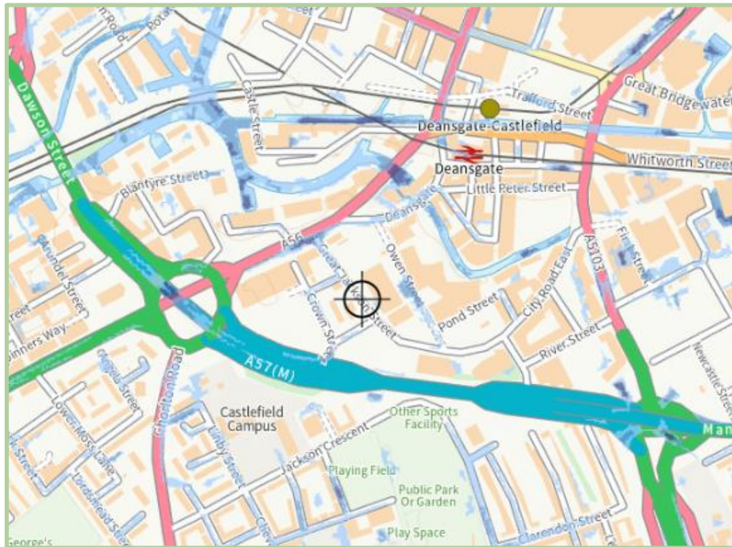
Figure 4.2 – Extent of Flooding from Surface Water
