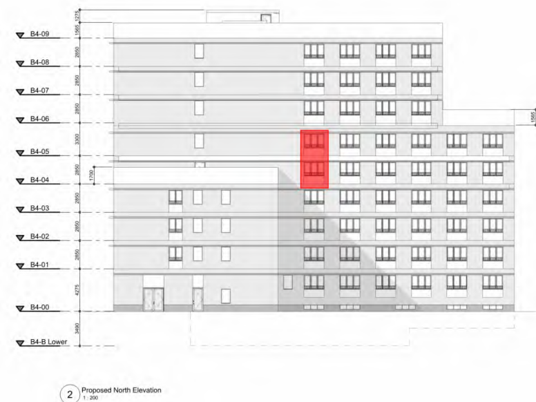
Figure 6 Block 4 north facade apartments where openable windows cannot be used at night to remove excess heat
