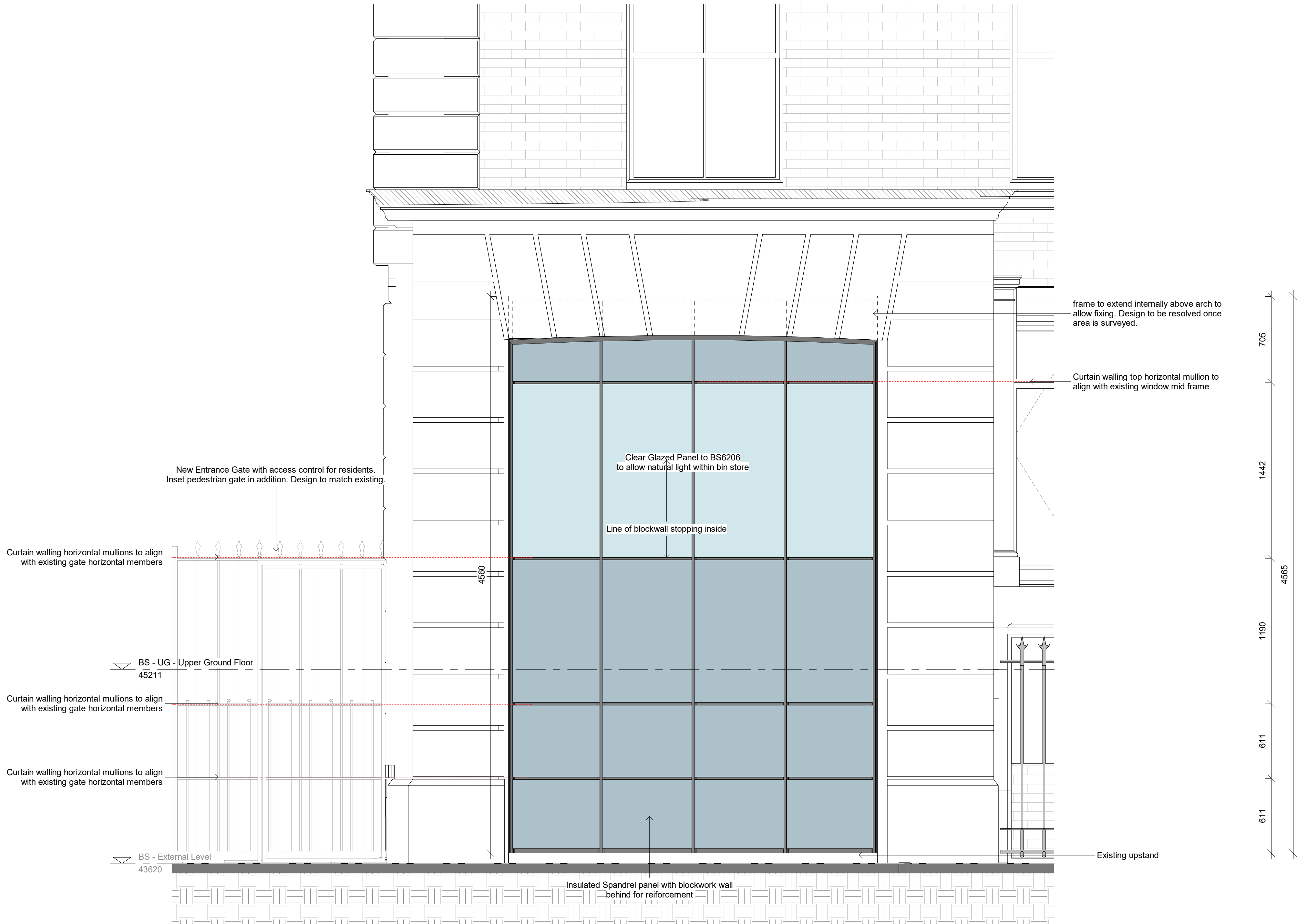
1 | Bin Store Curtain Wall - Elevation Copy 1
