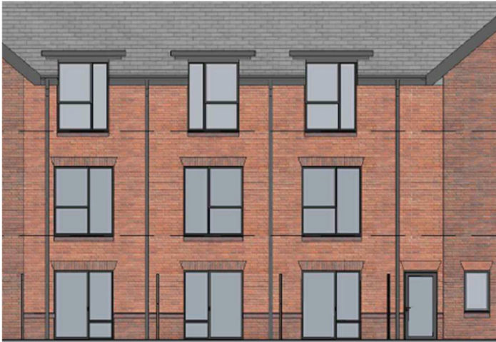
Figure Five: Previous East elevation showing access door leading from stair core and bedroom windows positioned unequally.
