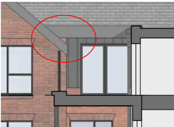
Figure Twelve: Previous Eaves design shown protruding over balcony.
