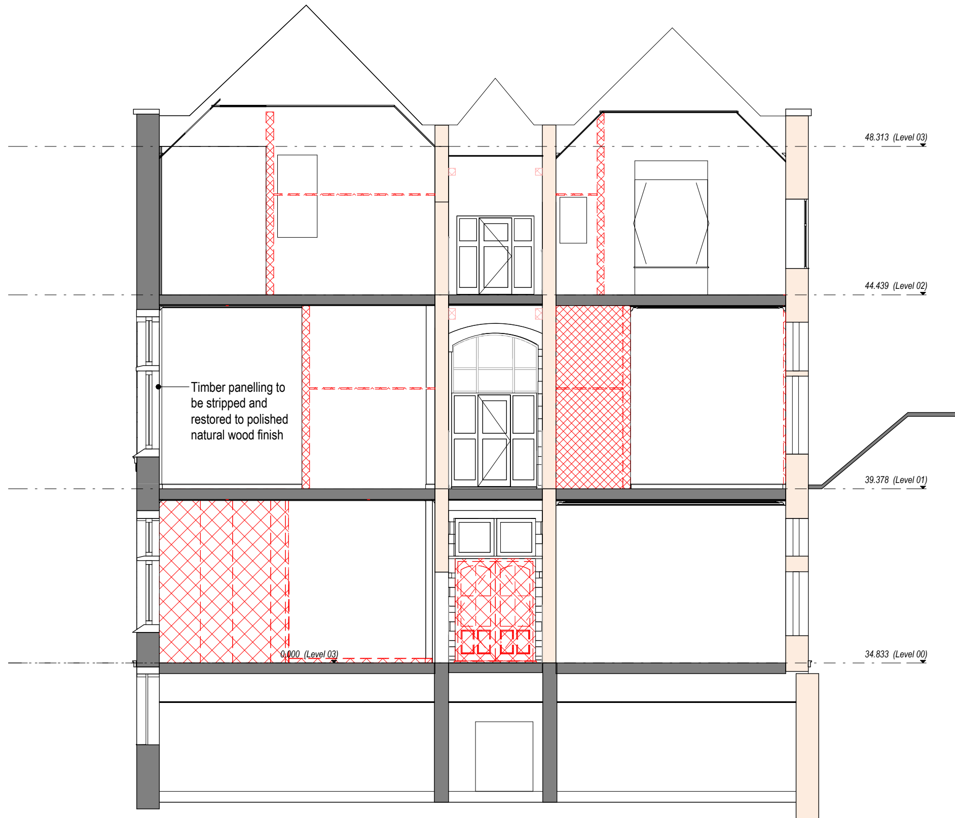
1 Proposed Demolition - GA Section 01 1 : 100
