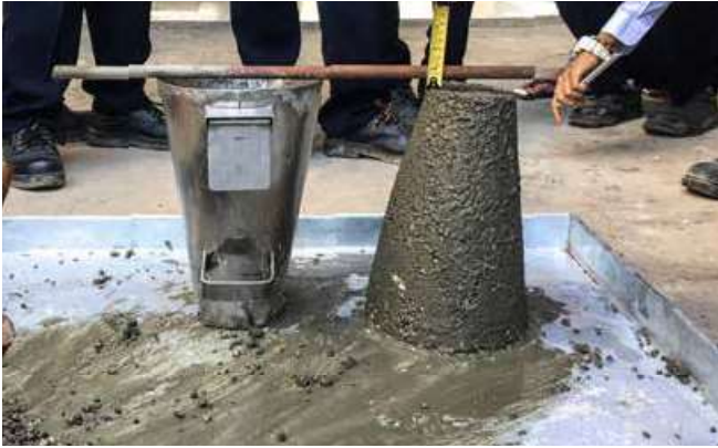
Slump test - Test moisture content of drycast concrete
