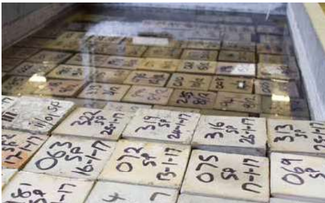
Concrete cubes - curing process before testing
